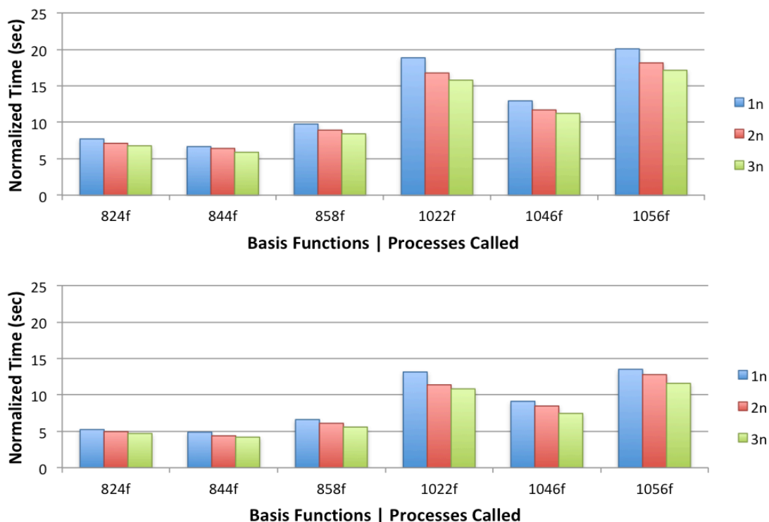
Figure 12. Normalized total execution times for semi-direct MP2 gradients for all six chemical systems tested at all three levels of oversubscription. The top represents two nodes and the bottom represents three nodes.
